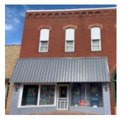
DM had new roofs and guttering installed, tuckpointed the front façade, canopy repaired, façade painting and rebuilt a portion of a masonry wall to get the building structurally sound and watertight. In conjunction with the Marceline Rotary organization, volunteers spent numerous hours removing water damaged ceilings, wall coverings and floorings.
